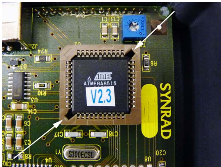
Figure 2 – Detail of chip extraction slots
