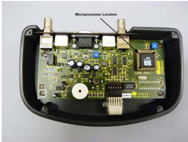
Figure 1 - View of control board mounted inside the Controller housing
