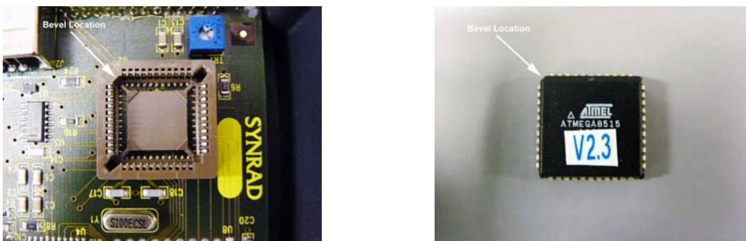
Figure 3 – Detail of bevels on chip and chip socket
