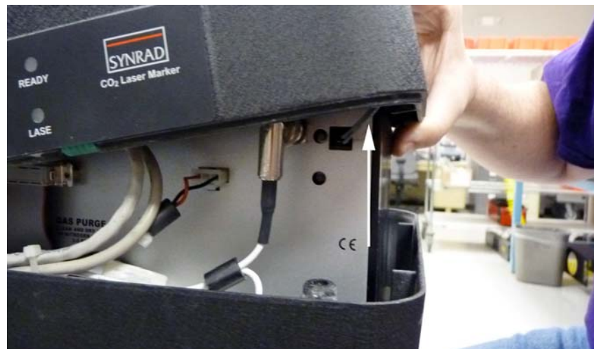
Figure 15 Two-wire cable positioning
