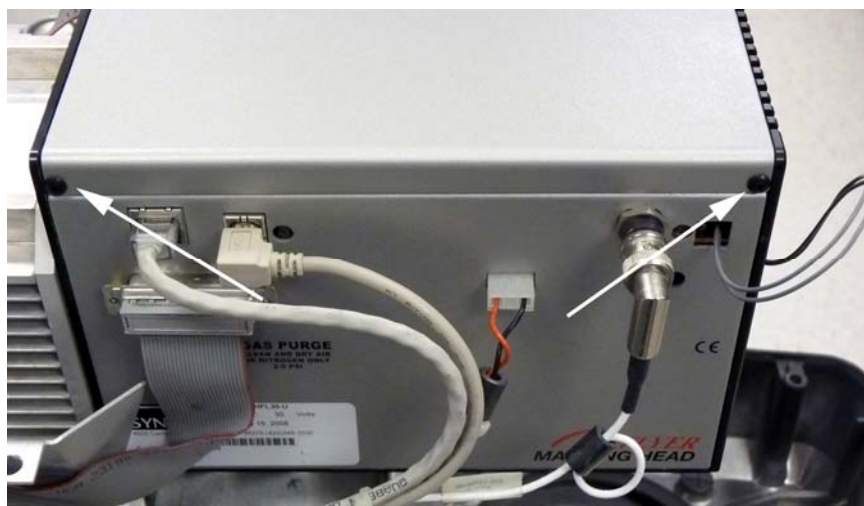
Figure 8 Side fasteners for Flyer cover
