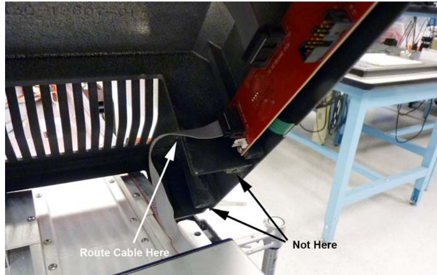
Figure 14 Ribbon cable positioning
