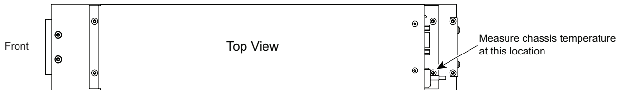
Figure 7 Firestar vi30 external temperature monitoring point
