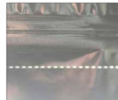
**Perforating** - requires a laser with high peak pulse power and excellent beam quality for crisp, symmetrical perforations. Recommended lasers include the **p Series.**
