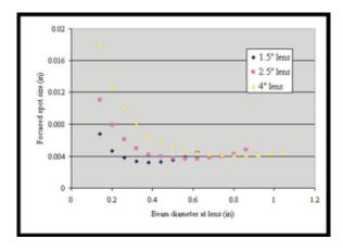
This graph shows the relationship between beam diameter and focused spot size for a number of standard lens focal lengths. If a flying optics system moves more than 0.5 m, the focused spot can be effected by around 5-25%, depending on the lens used. The graph is for a plano-convex shaped lens, and shows that as beam size increases, a point occurs when aberration effects become dominant.
