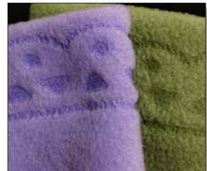
**Pattern Engraving** - requires a laser with higher continuous power and fast rise/fall times to avoid discoloration and charring. Recommended lasers include the **ti Series, f Series, and i Series**.
