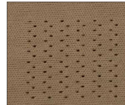
**Perforating for Breathe-ability** - requires a laser with higher peak power and fast rise/fall times to avoid discoloration and charring. Recommended lasers include the **p Series**.
